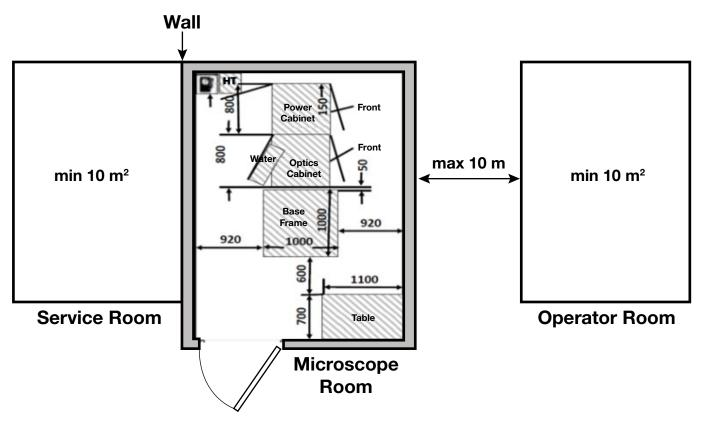
Figure 3. Recommended room layout for Talos L120C. The indicated dimensions are in millimeters.
