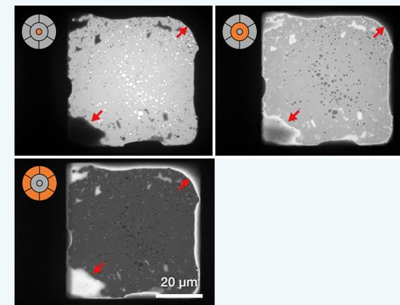
Figure 23. BF (top left), DF (top right), and HAADF (bottom left), images of a large-scale overview of one of the meshes. The images were acquired in wet mode, and liquid water is visible at the edges of the copper mesh (see red arrows).
