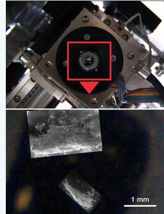
Figure 40. View of Maps Software's user interface showing the presence of two different datasets acquired on each fragment. The image on the bottom shows the overlay of the navigation camera image and the two acquired tile sets.
