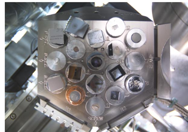
Figure 2. Top view of the multipurpose sample holder.
