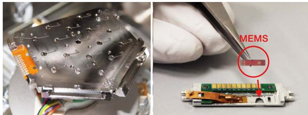
Figure 30. Multi-purpose sample holder with slot for microelectromechanical systems (MEMS)-based μHeater Holder cartridge.
