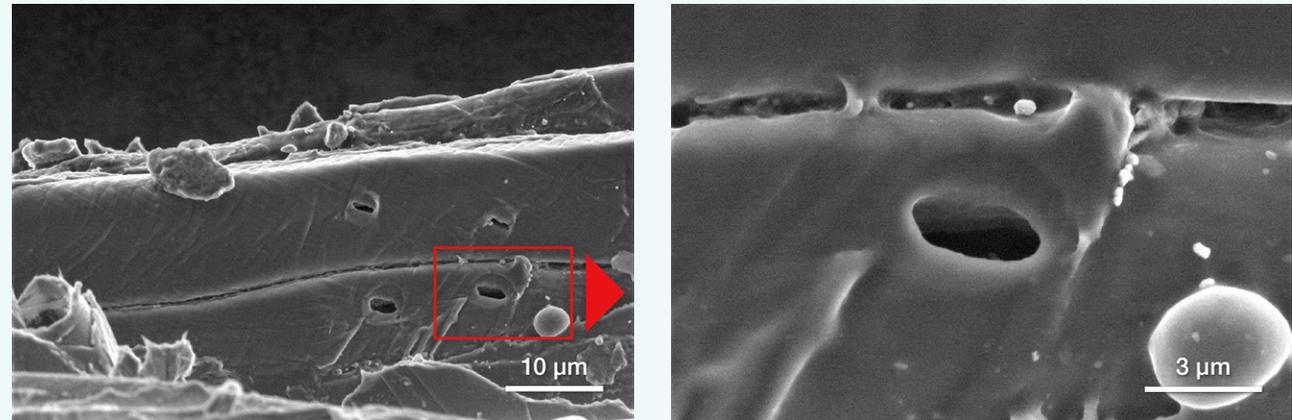
Figure 41. SE images from one of the two fragments, acquired on the fully hydrated sample (pressure 700 Pa, RH around 100%). The right image shows the presence of a water droplet. *Sample courtesy of Technische Universität Dortmund, Werkstoffe des Bauwesens, Germany*
