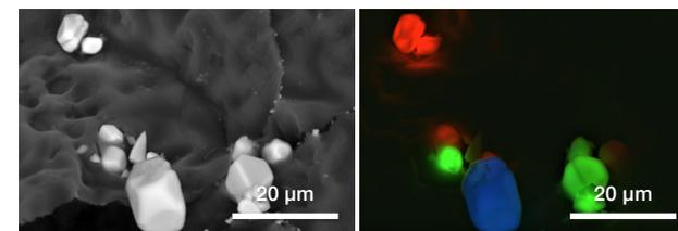
Figure 9. Red, green, and blue emitting particles from a cathode ray tube. Thanks to the information provided by the CLD detector, the different natures of these particles are easily seen, while the different emission properties were not visible by SEM imaging alone. (The compositional information provided by the DBS image on the left does not clarify the different nature of the particles.)
