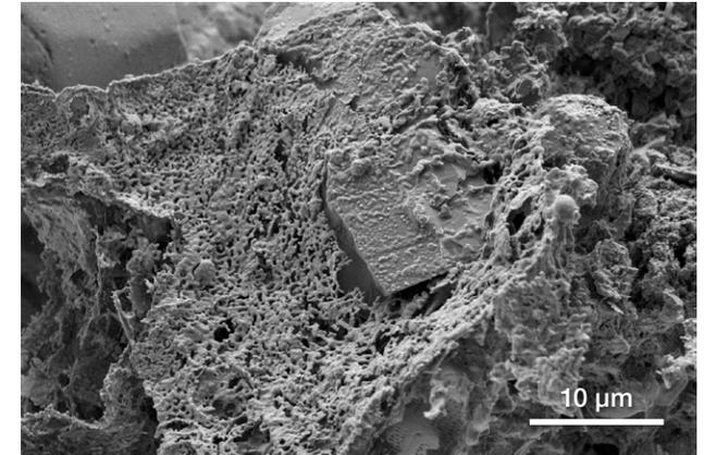
Figure 15. Diatoms and salt crystals in ash imaged with a pressure of 50 Pa. Acc voltage 3 keV.
