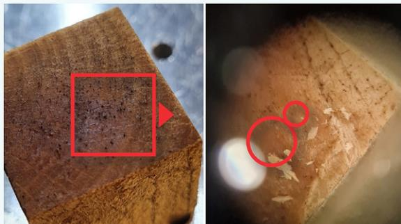
Figure 38. Wood sample. The highlighted fragments have been selected to be characterized.
