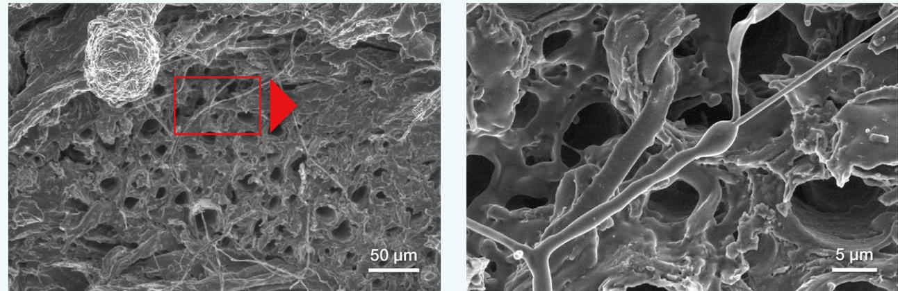
Figure 42. SE images from the second fragment, acquired on the fully hydrated sample (pressure 700 Pa, RH around 100%). The right image highlights a water-coated mycelium.
