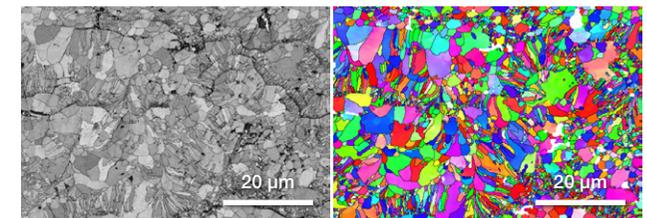
Figure 17. EBSD on zirconia from a thermal barrier coating. Acc voltage 15 keV, beam current 26 nA, pressure 100 Pa.
