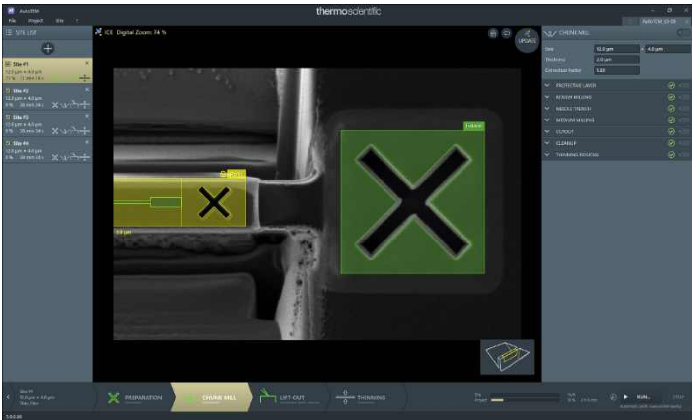
Figure 1. AutoTEM 5 software user interface: workflow steps at the bottom and settings on the right side. Intuitive UI with user guidance and instructive graphics helps to create highest quality samples for users with any experience level.
