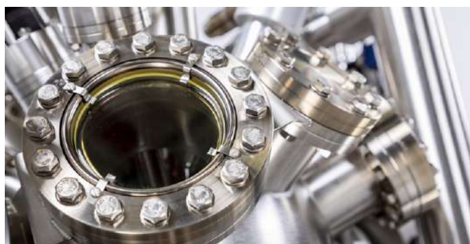
Figure 5: XPS UHV systems are typically manufactured from mu-metal or other magnetically shielded metal alloys. Parts are sealed onto the chamber using metal or polymer gaskets to ensure good vacuum.
