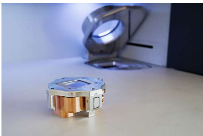
Figure 13: Nexsa G2 System vacuum transfer module for loading air-sensitive samples.
